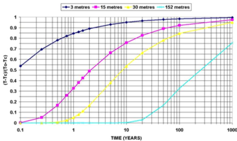
Figure 1: Variation of Temperature at the Centre of Reservoirs of Varying Thickness
